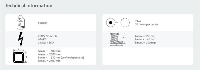
Technical data are valid for basic machine without options. Size according to layout.
