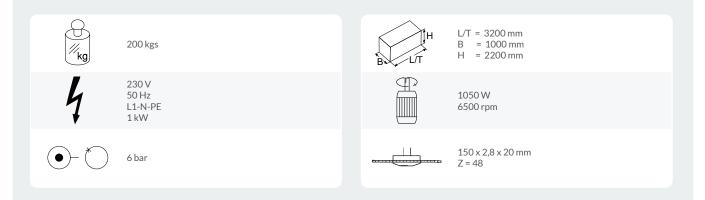
Technical data are valid for basic machine without options. Size according to layout.
